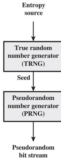
**Figure 7.2** Generation of Seed Input to PRNG
