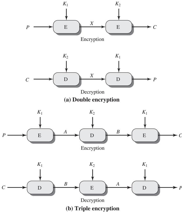
Figure 6.1 Multiple Encryption
