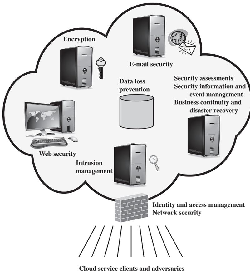
Figure 16.11 Elements of Cloud Security as a Service
