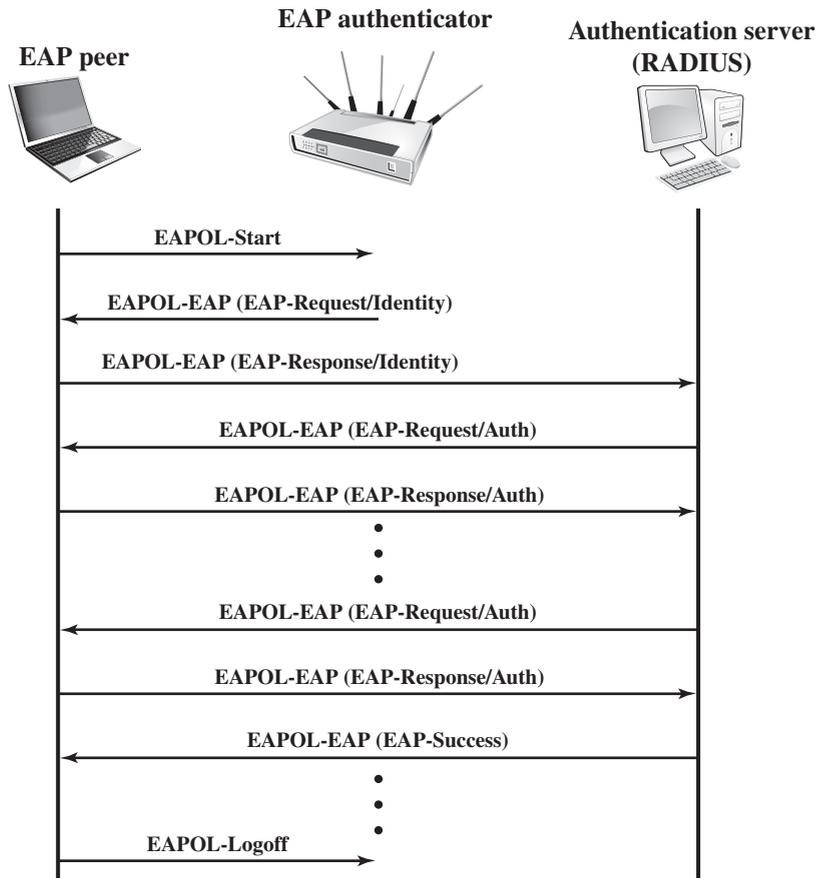
Figure 16.6 Example Timing Diagram for IEEE 802.1X
