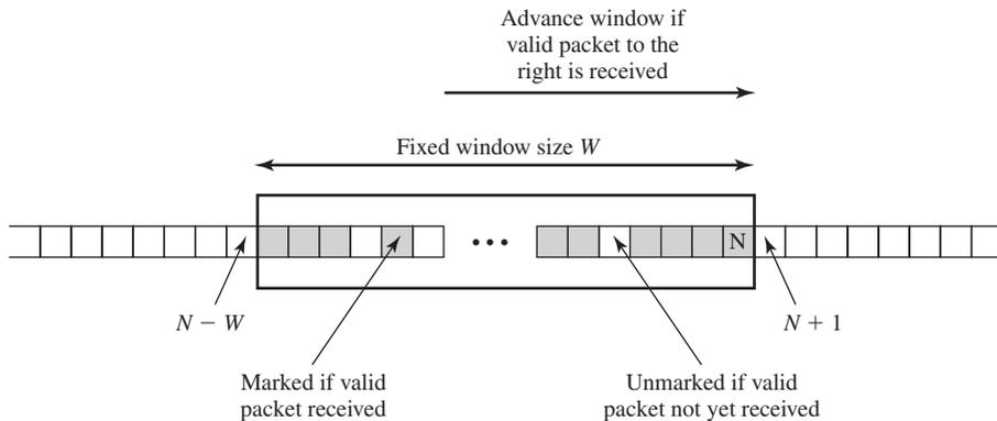
**Figure 20.6** Anti-replay Mechanism
