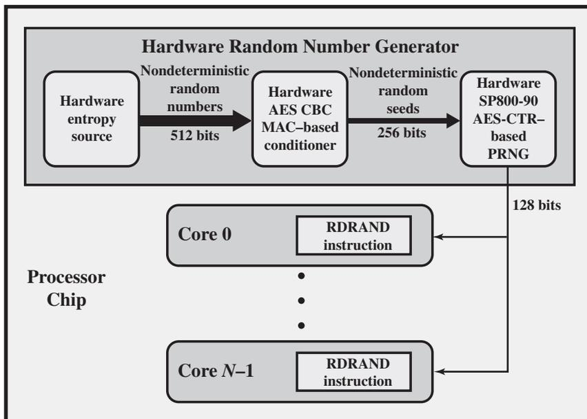
Figure 7.9 Intel Processor Chip with Random Number Generator
