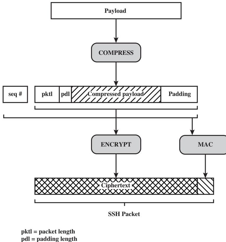
**Figure 17.10** SSH Transport Layer Protocol Packet Formation
