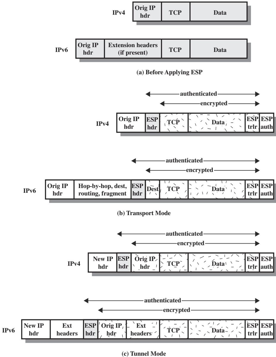
Figure 20.8 Scope of ESP Encryption and Authentication
