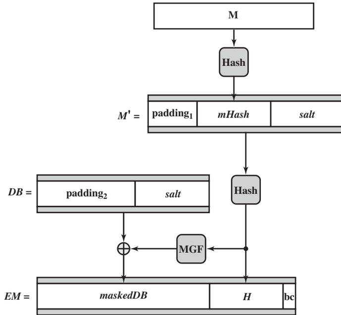
Figure 13.7 RSA-PSS Encoding
