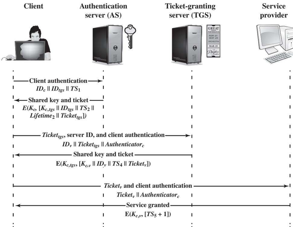
Figure 15.2 Kerberos Exchanges
