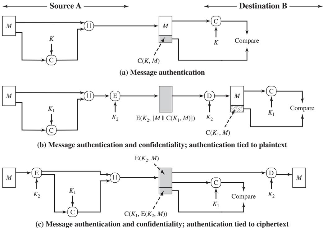
Figure 12.4 Basic Uses of Message Authentication code (MAC)
