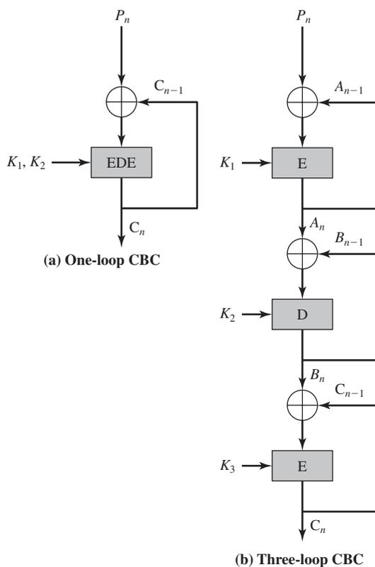
Figure 6.12 Use of Triple DES in CBC Mode
