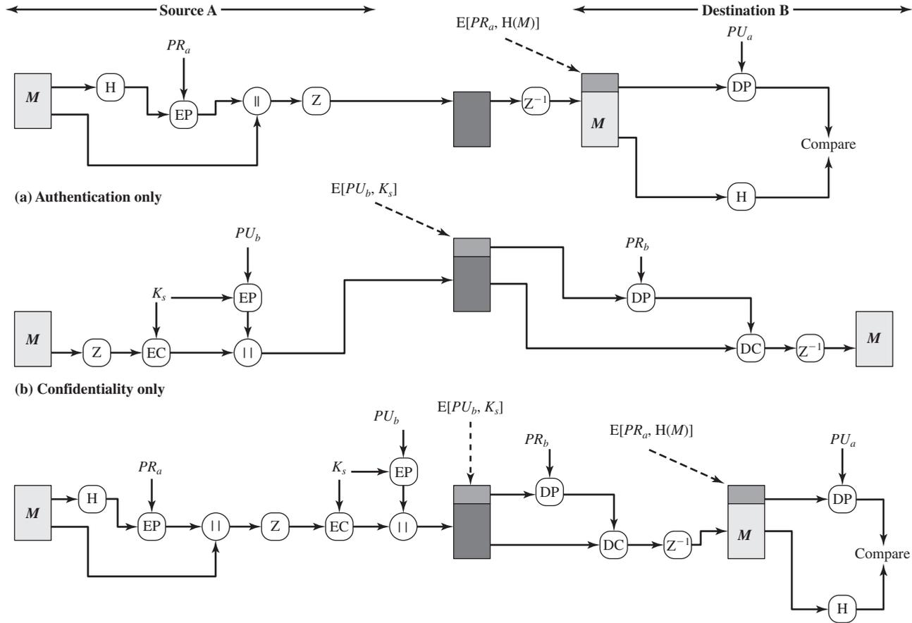
Figure 19.1 PGP Cryptographic Functions
