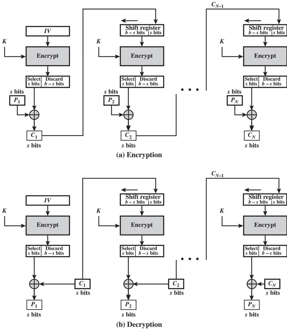
Figure 6.5  $s$ -bit Cipher Feedback (CFB) Mode
