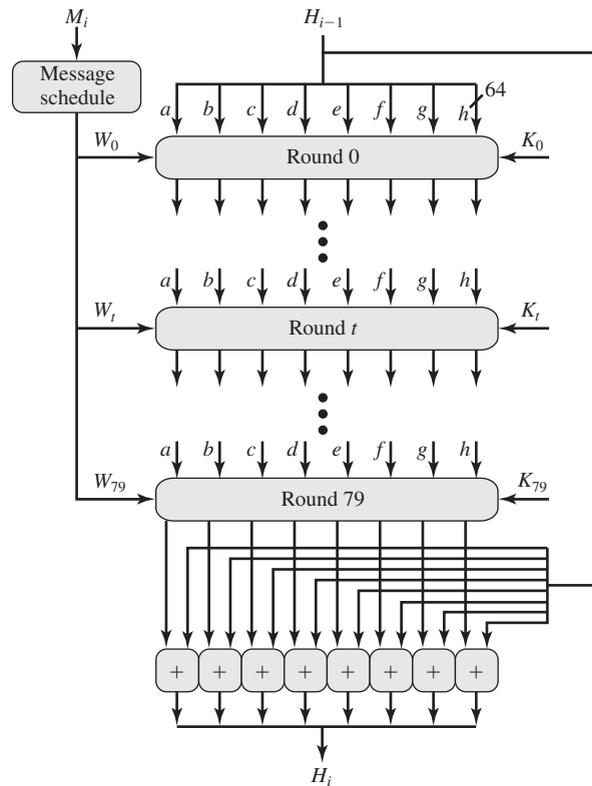
Figure 11.10 SHA-512 Processing of a Single 1024-Bit Block
