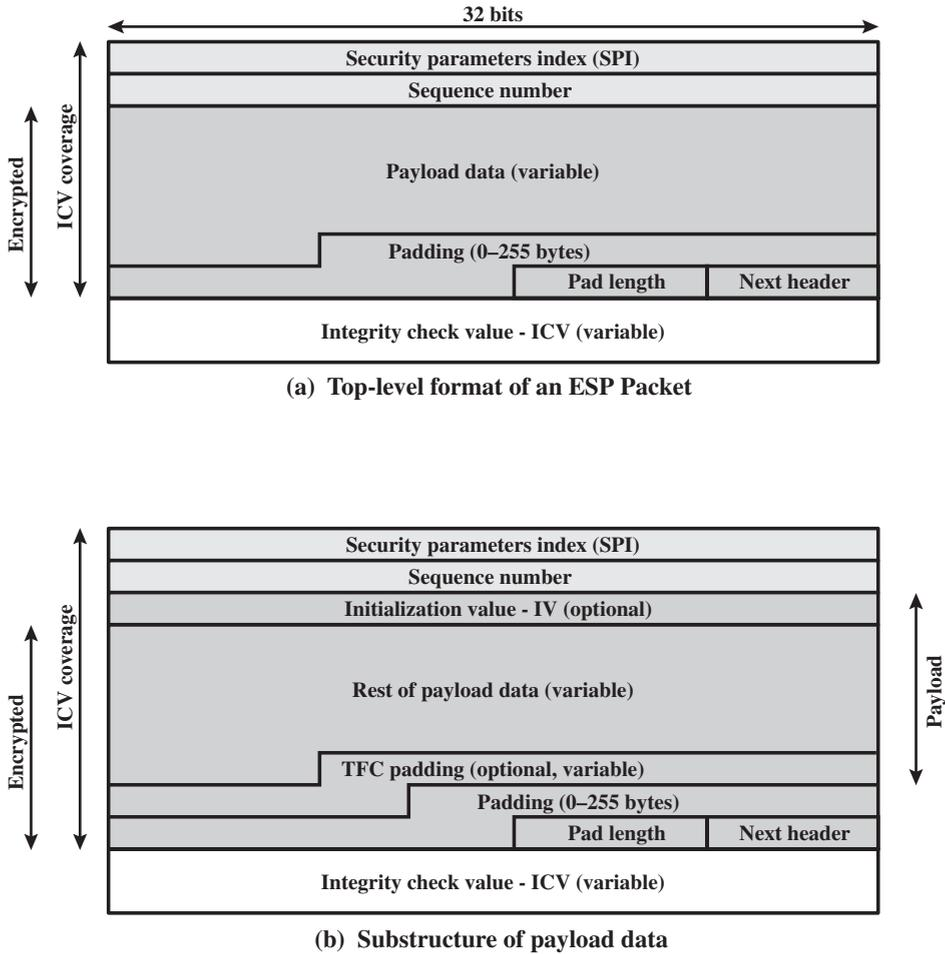
Figure 20.5 ESP Packet Format
