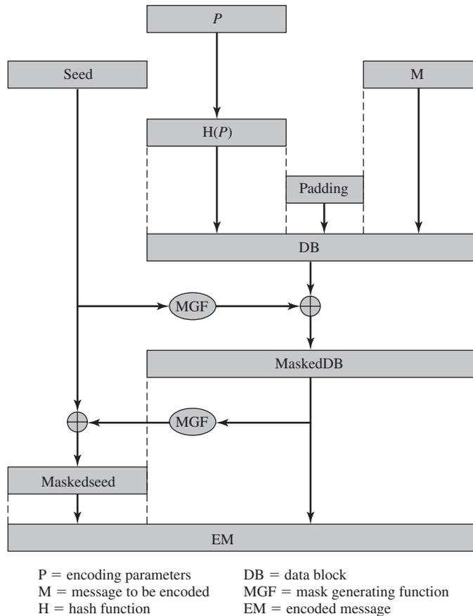
**Figure 9.10** Encryption Using Optimal Asymmetric Encryption Padding (OAEP)
