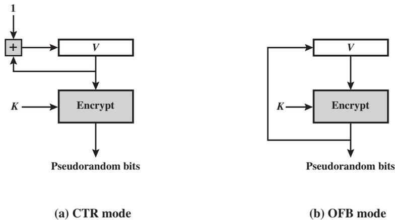
Figure 7.4 PRNG Mechanisms Based on Block Ciphers
