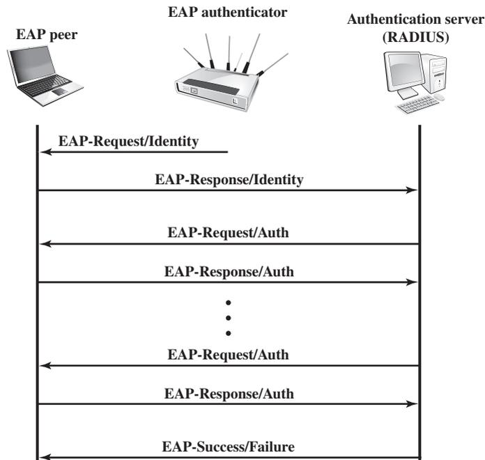
Figure 16.4 EAP Message Flow in Pass-Through Mode
