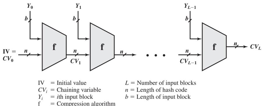
Figure 11.8 General Structure of Secure Hash Code
