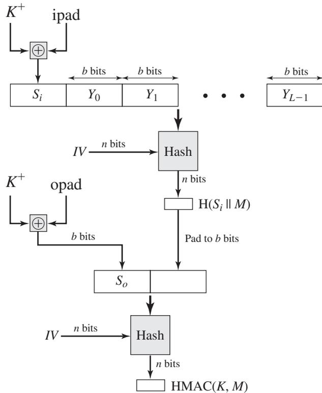
Figure 12.5 HMAC Structure
